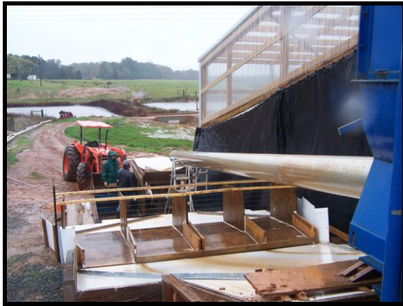
Figure 1. Test set-up, including mixing tank, supply pipe and wooden box with simulated area inlet inside collection tank.
