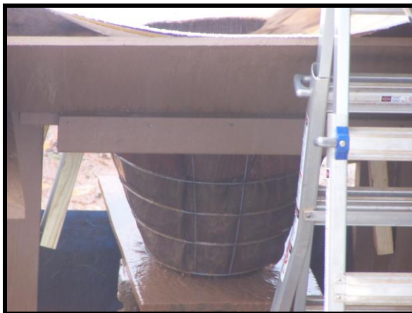
Figure 2. 200 SedCatch® Sediment Basket™ Collecting Sediments in Test
